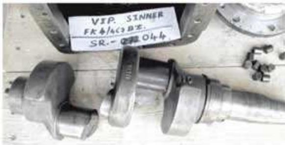
Figure 10c : Broken crankshaft.
