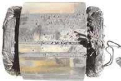
Figure 17 : Motor failure due to contaminants.
