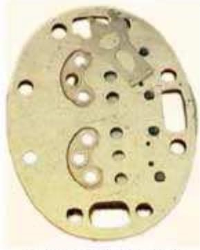
Figure 6 : Dry valve plate.
