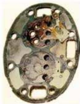
Figure 5 : Oily/Sludge valve plate.
