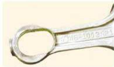
Figure 9 : Oblong small end of the connecting rod.
