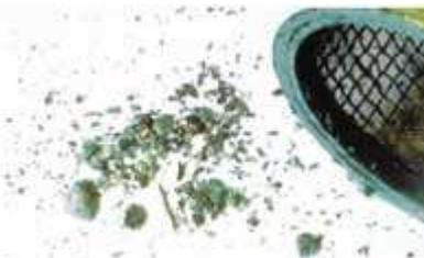
Figure 12b : Choked compressor suction strainer.
