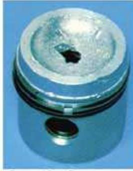
Figure 10b : Punched hole in the piston.
