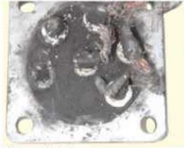
Figure 18 : Terminal box corroded.
