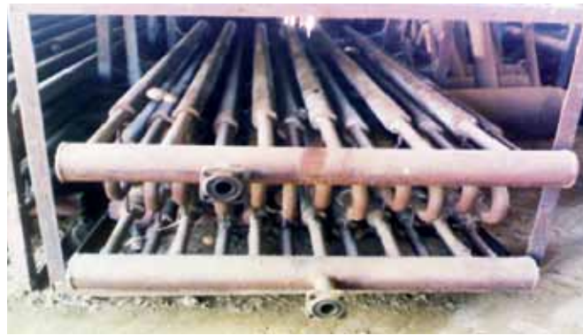
Figure 2: Ceiling suspended coils (bunker coils)
